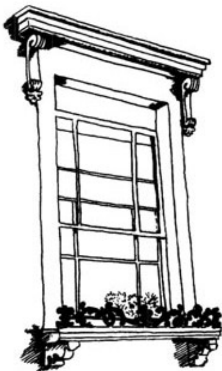
Historically correct timber sliding sash window with slim glazing bars (no horns), margin lights, internal shutters, ornate stucco architrave and brackets, and cast iron balconette
